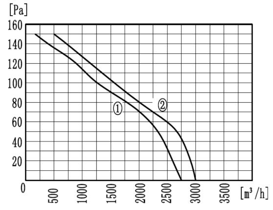
Curve 1: 50HZ Curve 2: 60HZ
